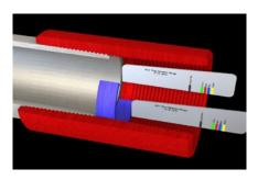
MLT Ring selection is made simply with a tool inserted into the end of the coupling.
