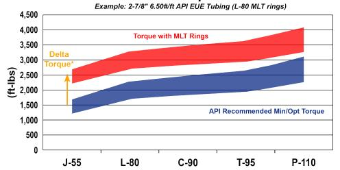
\*Delta Torque is the torque boost added to the normal make-up torque, referred to as "shoulder torque". Higher torques may be available with higher strength MLT rings.
