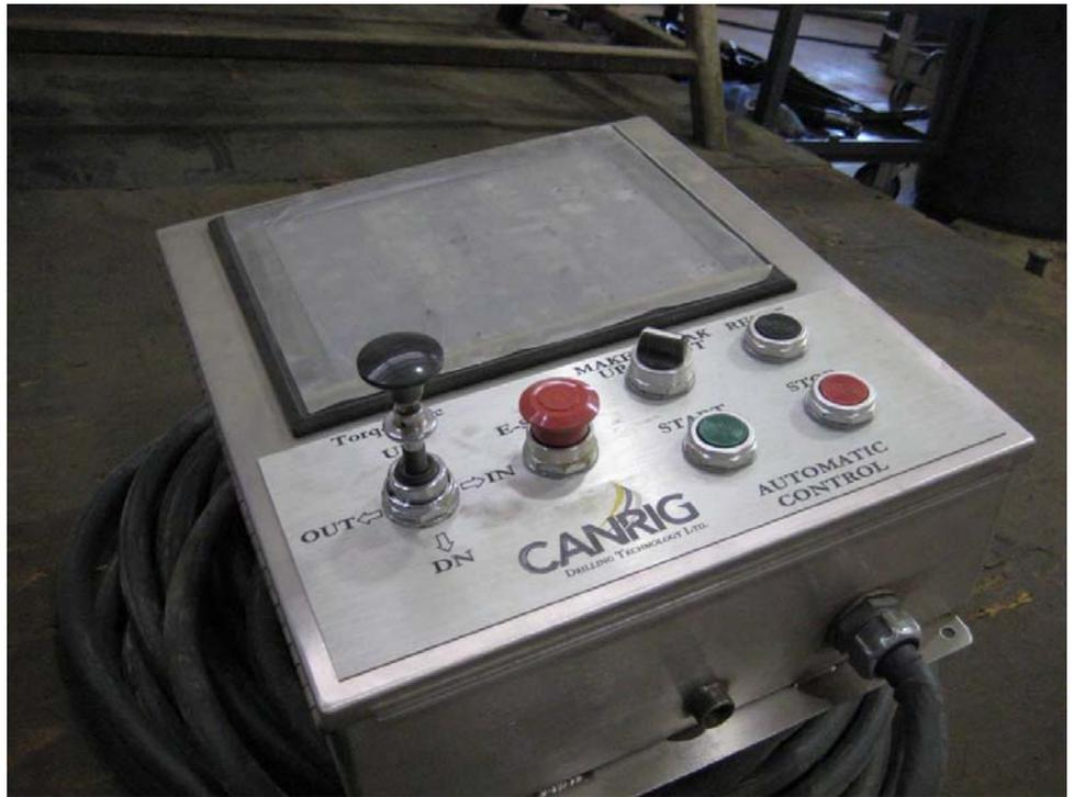
**Figure 2: New locking joystick**
