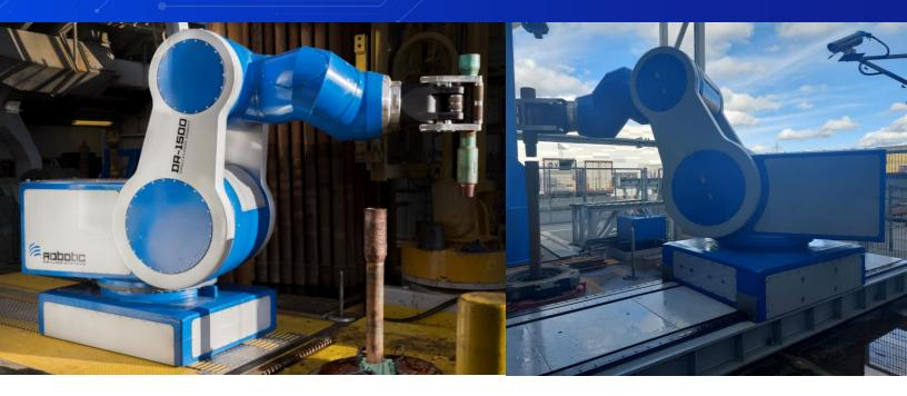
The fully electric Drill Floor Robot (DFR-1500) automates all pipe and tool operations to reduce the needs for manual labor on a rig's drill floor.
