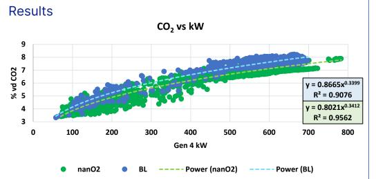
Over both testing periods, the graph above plots electrical kilowatts (ekW) versus  $CO_2$ % vapor density (vd). The nan $O_2$  trend line is lower in the  $CO_2$  throughout the whole load range recorded during the test. This verifies that the rig produces a lower percentage of  $CO_2$  for every given ekW power consumption, implying an overall reduction in  $CO_2$  emissions for any given level of work performed.
