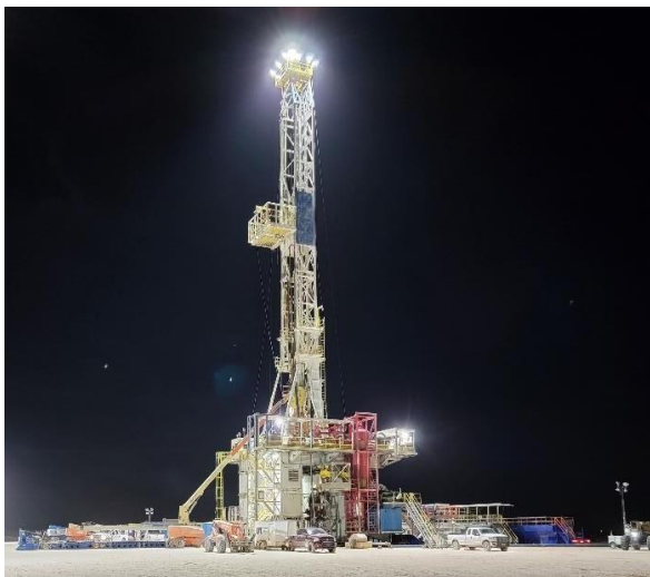
Each LED kit offers between 600K- 1M lumens with 2-to-4-foot candles in a 150' radius from the rig floor
