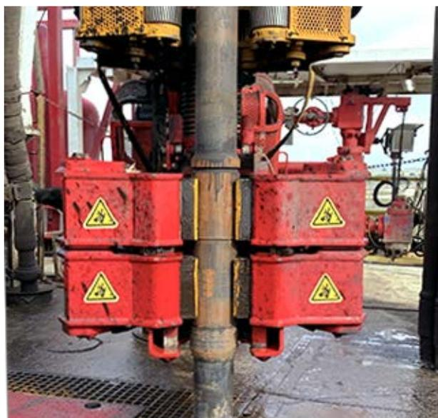
Figure 11: Tongs Aligned to Pipe Joint
