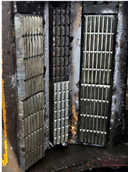
Figure 10: Dies Within Proper Wear
