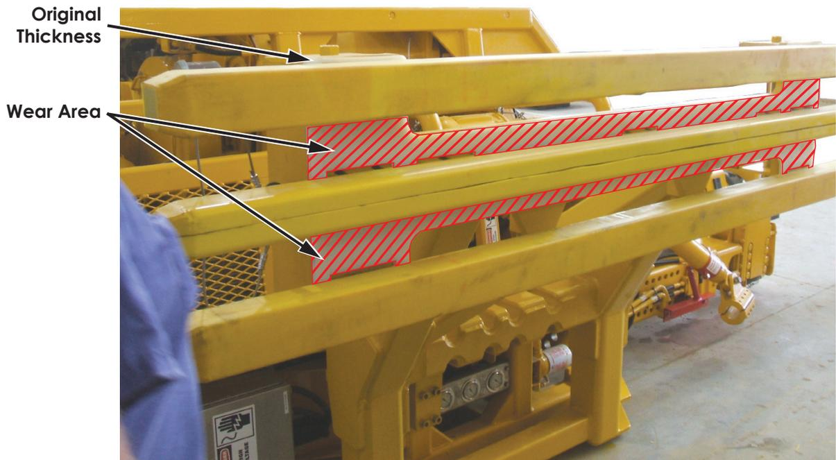
Figure 2: Measure Wear Pad in these Two Places
