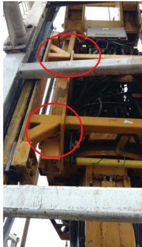
Figure 1: Frame Inspection Areas. Inspect Both Sides.
