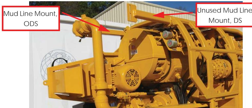
Figure 1: Remove the Unused ODS or DS Mud Line Mount
