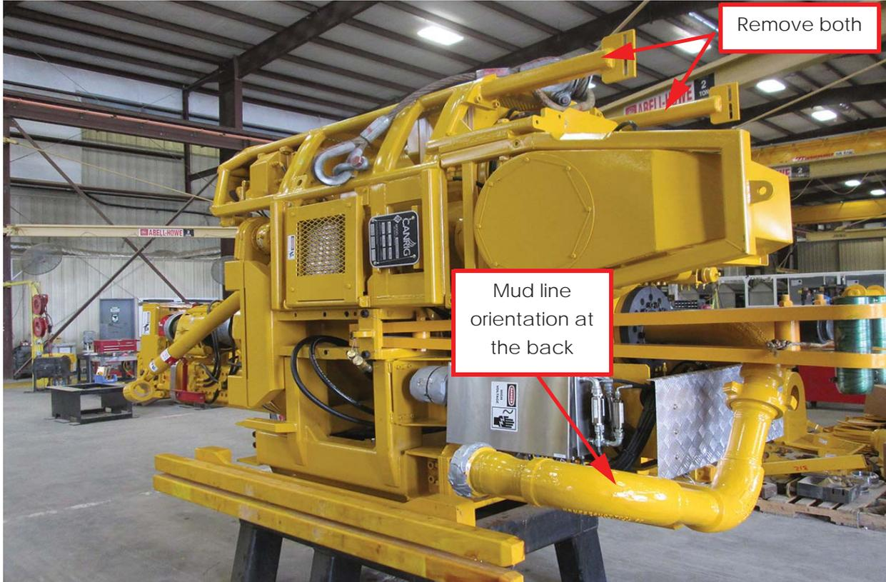
Figure 2: For top drives with the mud line orientation at the back of the top drive, remove both unused mud mounts and fasteners
