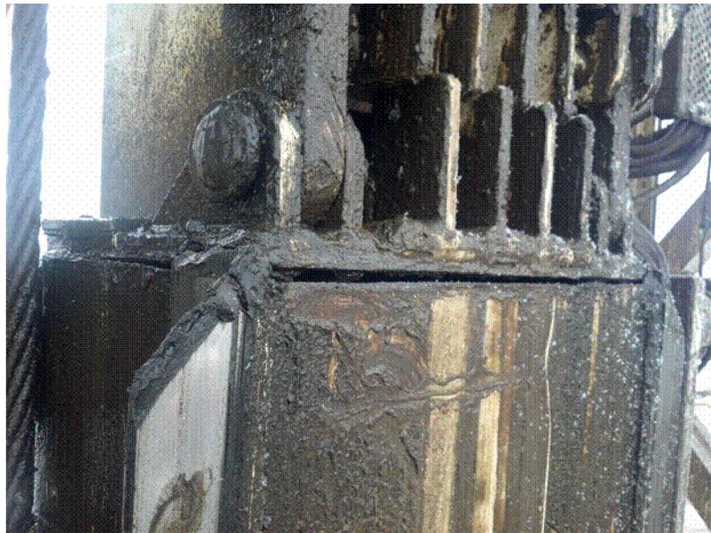
Figure 1: Cracked Portable Torque Guide Weld Joint
