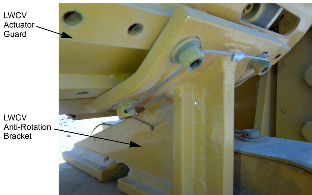
Figure 1: LWCV Anti-Rotation Bracket with Safety Wire in Place
