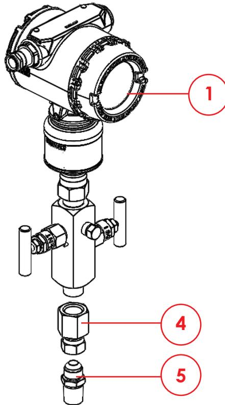
Figure 3: Transmitter assembly (with JIC fittings)
