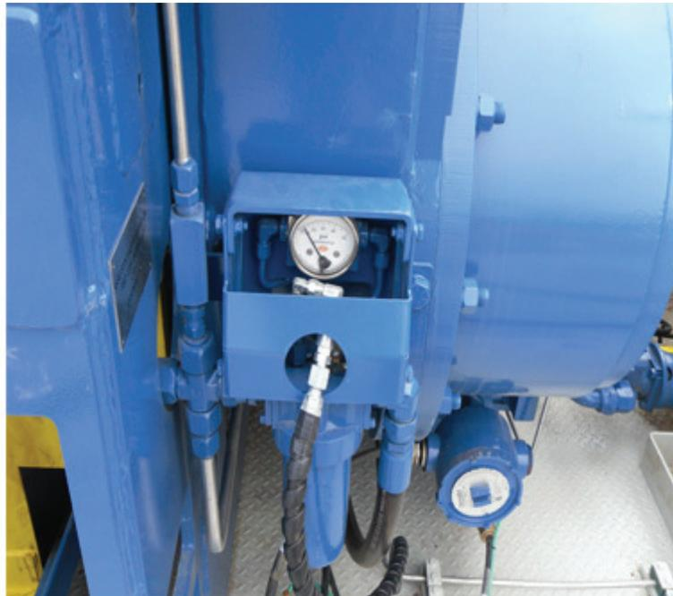
Figure 1: Old Lube Filter Assembly
