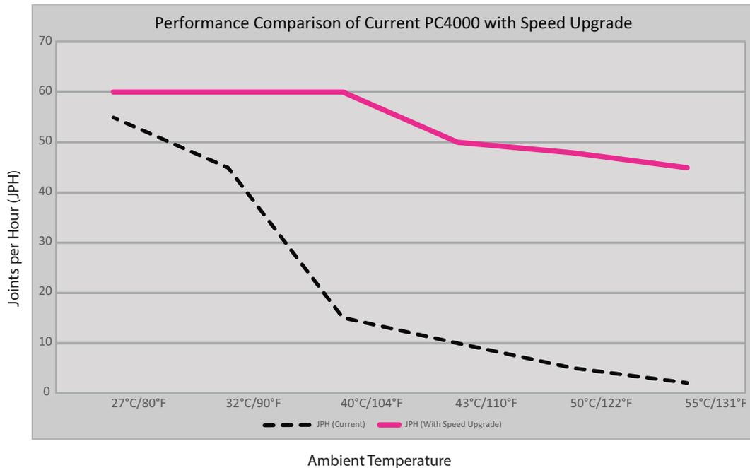
Figure 1: Current PC4000 Design Performance Compared with PC4000 Equipped with Speed Upgrade Kit AY52027 and latest PLC and HMI Upgrade
