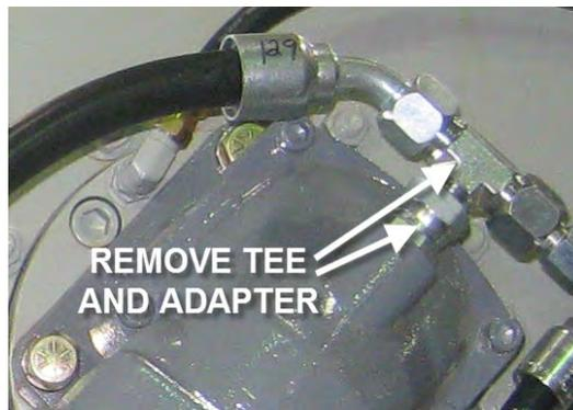
Figure 1: Adapter and Tee Fitting
