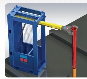
Keeping drill pipe centered is an important factor when mitigating damage to connections and external pipe equipment, such as clamps and cables, while tripping pipe.
