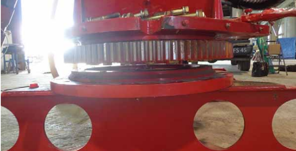
Figure 8: Disconnected bottom plate.
